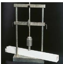
Apparatus for shock testing at low temperature.
