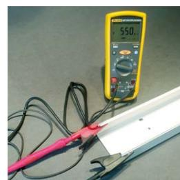
Apparatus for insulation resistance above 100 MΩ.
