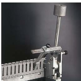
Apparatus for finger-removal and side-segment removal test.
