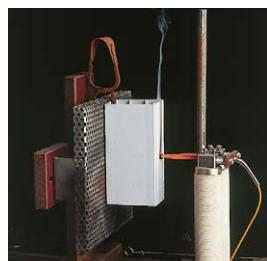
Apparatus for testing heat resistance (850°C) GWT.
