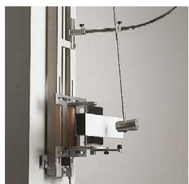
Apparatus for shock testing at room temperature.
